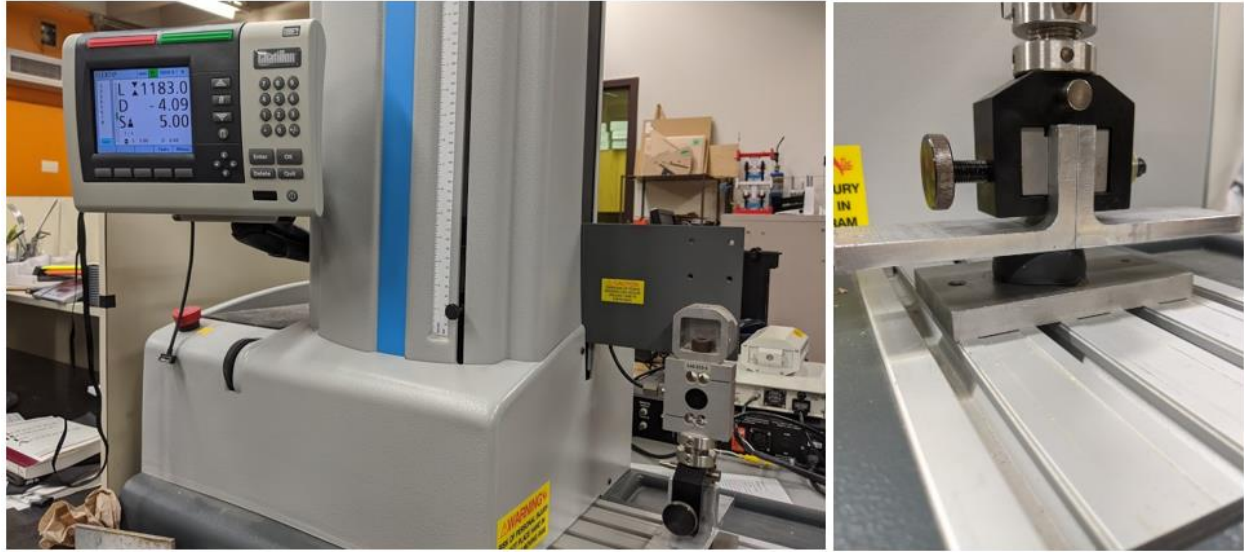
Figure 18: Rubber cane tip material testing
