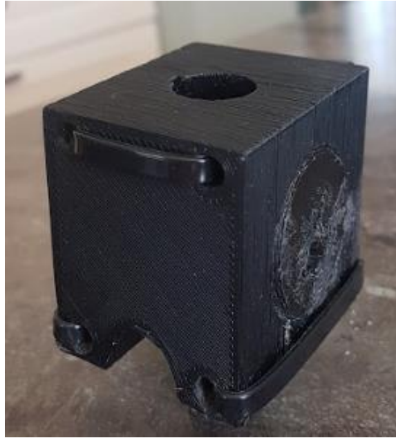
Figure 35: 3D printed cylindrical cover and cylindrical shaft end
